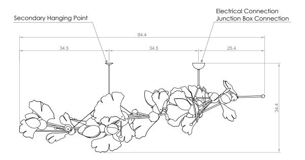
1) Locate secondary hanging hub and hardware. Insert hanging cables into cable gripper hardware on fixture frame. Cable lengths are marked to final depth with tape label.
