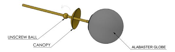
1) Unscrew ball finial and carefully slide back, releasing the fitter canopy.
