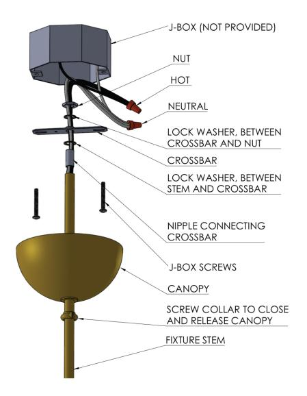
4) Prepare the junction box to receive the cross bar.
